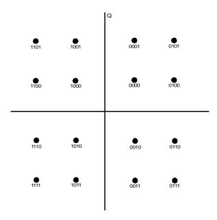
Figure 152—16-QAM constellation (gray-coded)
