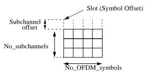
Figure 215—Example of the data region which defines the OFDMA allocation
