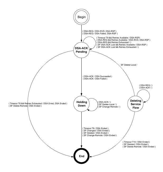
Figure 101—DSA—Remotely Initiated Transaction state transition diagram
