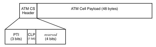
Figure 5—CS PDU format for VC-switched ATM connections
