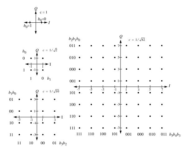
Figure 203—BPSK, QPSK, 16-QAM, and 64-QAM constellations
