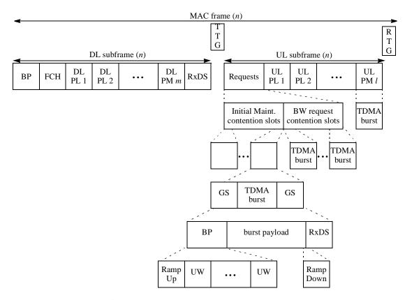
Figure 193—Example of TDD frame format
