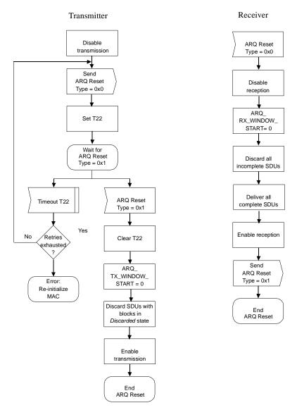
Figure 34—ARQ Reset message dialog—transmitter initiated
