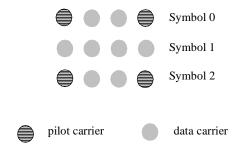
Figure 236—Description of an uplink tile
