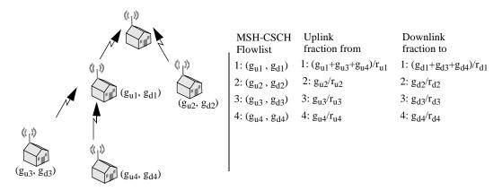
Figure 42—MSH-CSCH flow usage example
