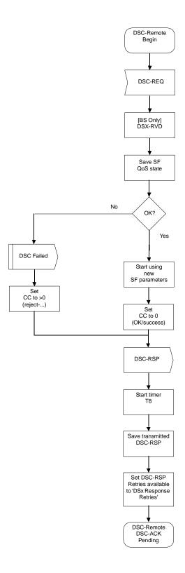
Figure 120—DSC—Remotely Initiated Transaction Begin state flow diagram
