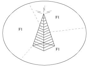
Figure B.5—Reuse of 1 configuration, 3 sectors per cell
