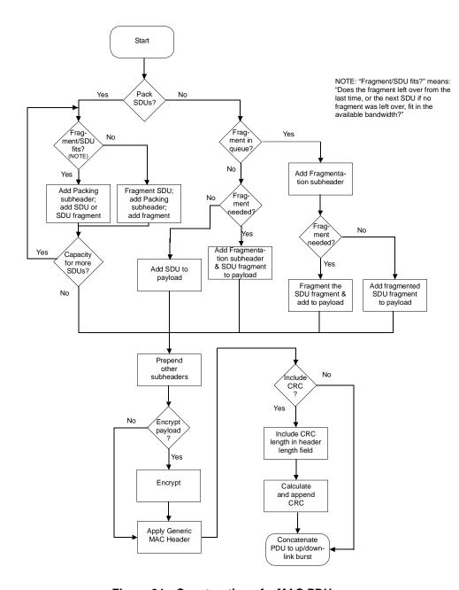
Figure 24—Construction of a MAC PDU
