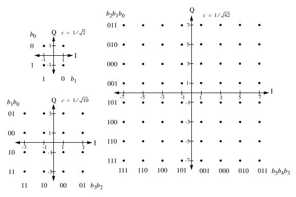
Figure 263—QPSK, 16-QAM, and 64-QAM constellations
