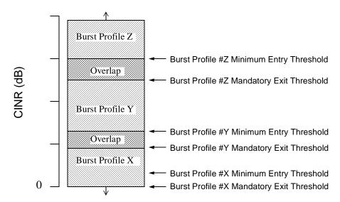
Figure 81—Burst profile threshold usage
