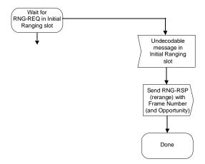
Figure 64—Initial ranging—BS response to undecodable message
