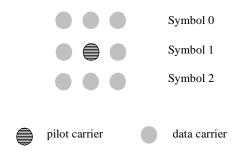
Figure 237—Description of an uplink tile
