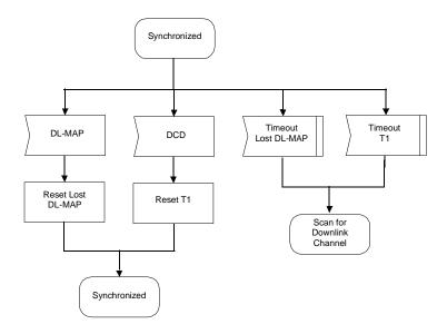
Figure 57—Maintaining downlink synchronization
