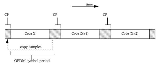
Figure 242—Periodic-ranging or bandwidth-request transmission for OFDMA using three consecutive codes
