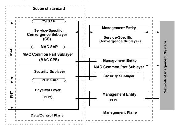
Figure 1—IEEE Std 802.16 protocol layering, showing SAPs
