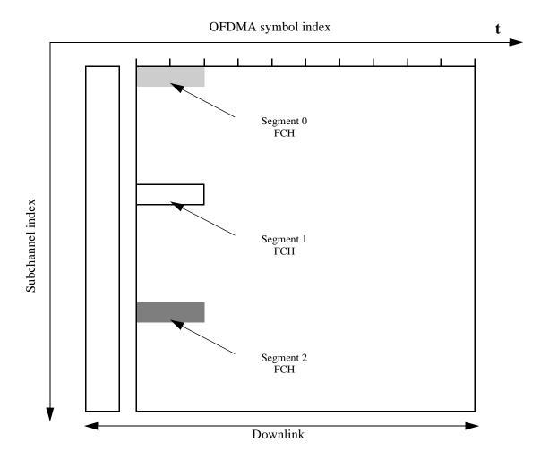
Figure 220—FCH subchannel allocation for all 3 segments
