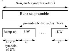
Figure 179—Burst set preamble composition
