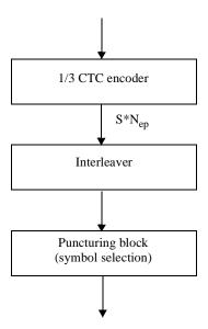
Figure 258—Block diagram of subpacket generation
