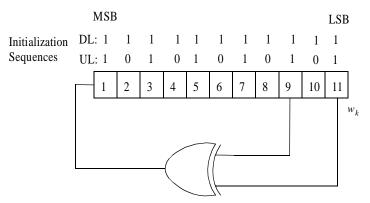
Figure 262—PRBS for pilot modulation
