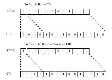
Figure 22—Reduced CID Decoding
