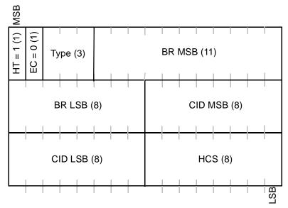
Figure 20—Bandwidth request header format
