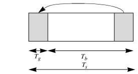
Figure 213—OFDMA symbol time structure
