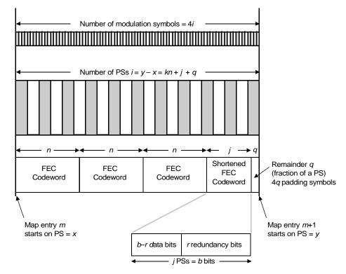
Figure 142—DL-MAP usage with shortened FEC blocks—TDM case
