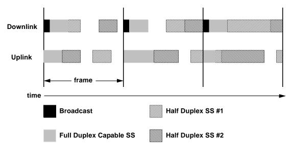
Figure 44—Example of Burst FDD bandwidth allocation
