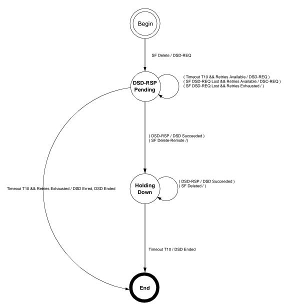
Figure 104—DSD—Locally Initiated Transaction state transition diagram
