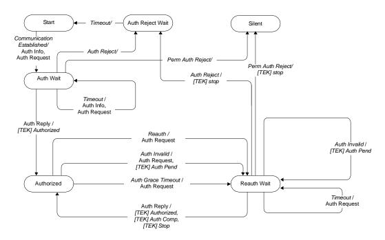
Figure 131—Authorization state machine flow diagram
