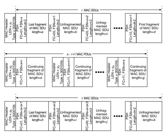
Figure 28—Packing with fragmentation
