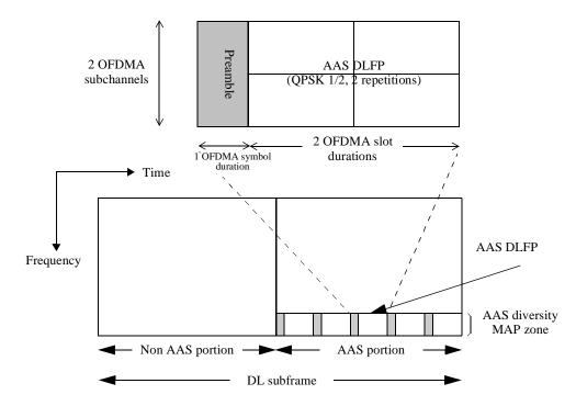
Figure 223—Example of allocation for AAS\_DL\_Scan IE
