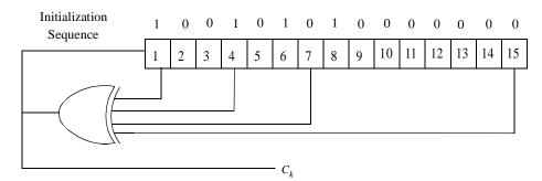
Figure 243—PRBS for ranging code generation
