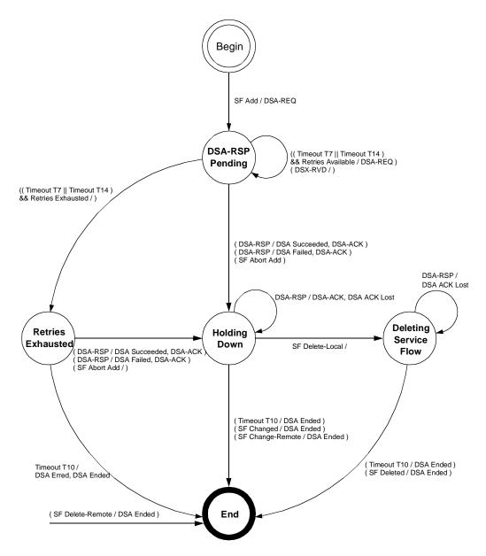
Figure 100—DSA—Locally Initiated Transaction state transition diagram
