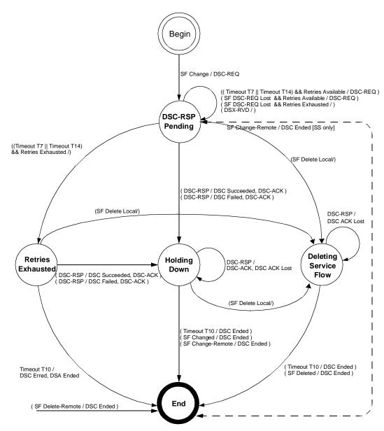
Figure 102—DSC—Locally Initiated Transaction state transition diagram
