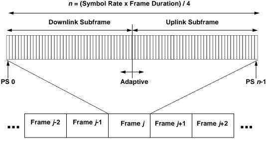
Figure 139—TDD frame structure
