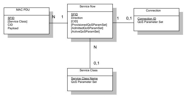
Figure 95—Theory of Operation Object Model
