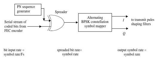
Figure 176—Spread BPSK processing
