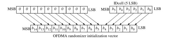
Figure 261—Initialization construction for the PRBS of the randomizer
