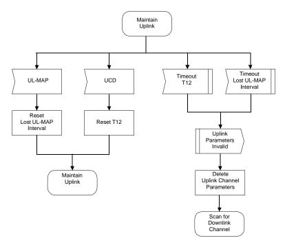
Figure 59—Maintain uplink parameters
