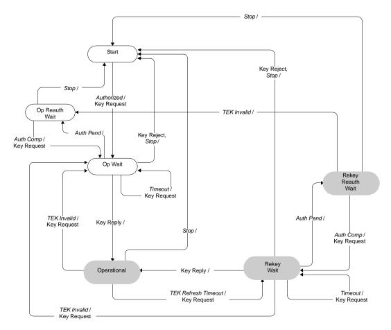
Figure 132—TEK state machine flow diagram
