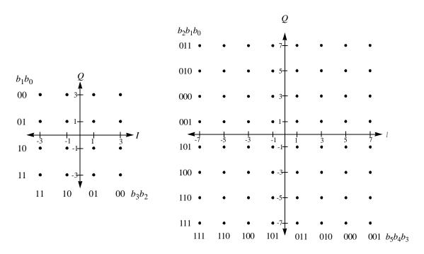
Figure 174—Pragmatic maps for 16-QAM and 64-QAM constellations
