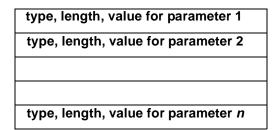
Figure 267—Create TLV entries for parameters required by the SS
