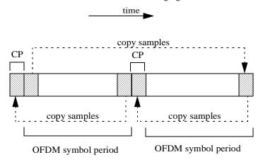
Figure 239—Initial-ranging transmission for OFDMA
