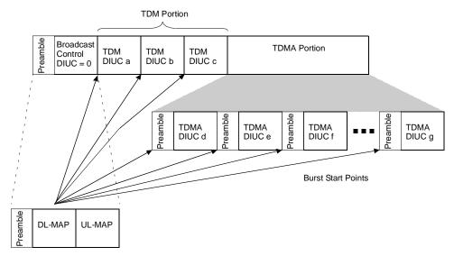
Figure 141—FDD downlink subframe structure
