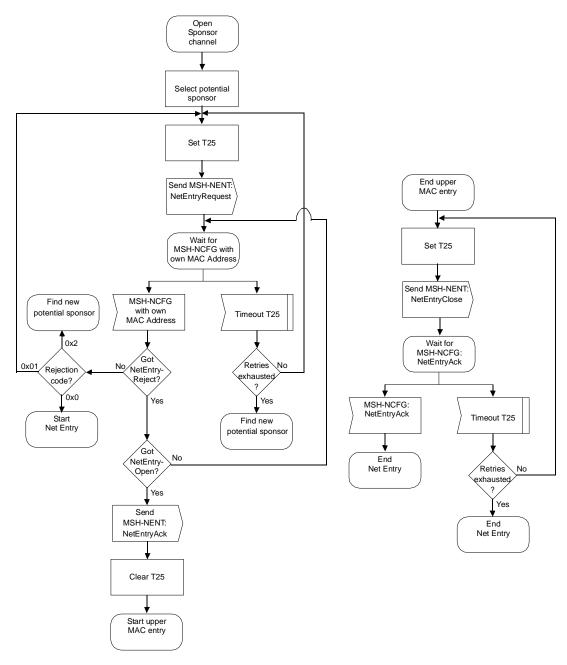
Figure 74—Mesh network synchronization and entry—New node—II
