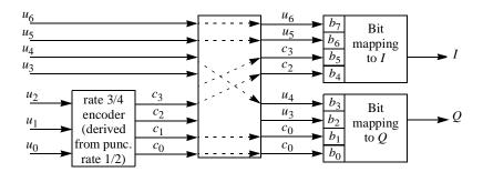
Figure 167—Optional pragmatic TCM encoder for rate 7/8 256-QAM
