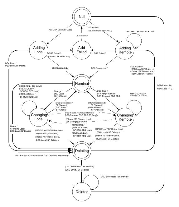
Figure 99—Dynamic Service Flow state transition diagram
