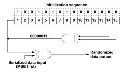
Figure 146—Randomizer logic diagram
