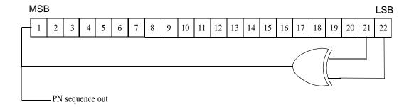
Figure 177—Spreading PN sequence generator
