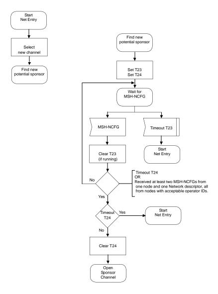
Figure 73—Mesh network synchronization and entry—New node—I
