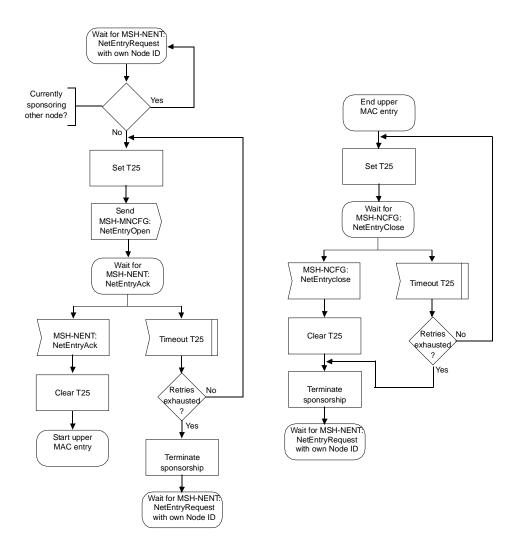
Figure 75—Mesh network synchronization and entry—Sponsor node
