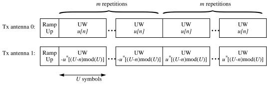
Figure 184—STC burst set preamble
