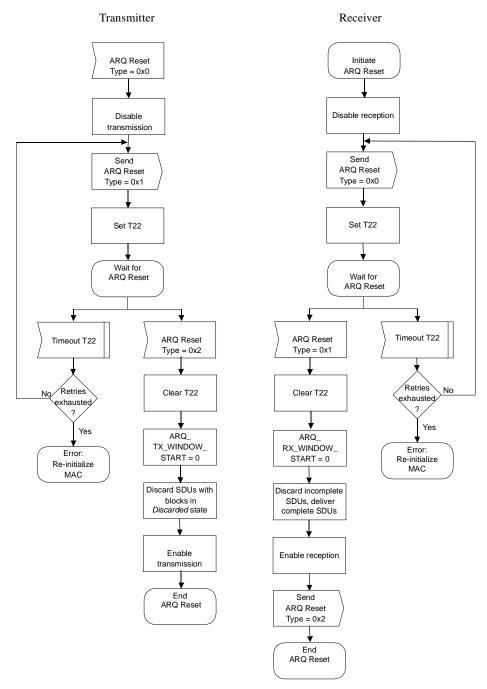
Figure 35—ARQ Reset message dialog—receiver initiated
