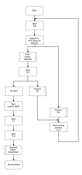
Figure 56—Obtaining downlink synchronization
