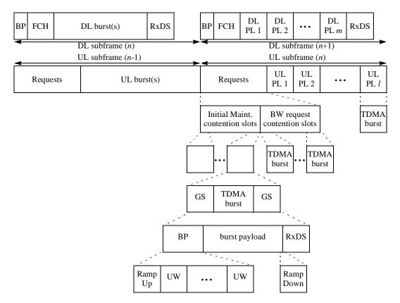
Figure 192—Example of FDD frame format
