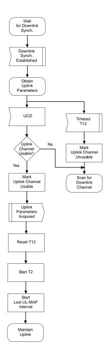
Figure 58—Obtaining uplink parameters
