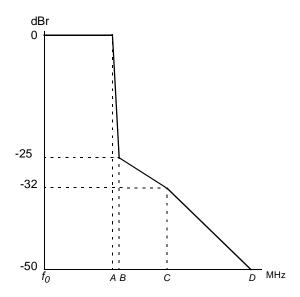
Figure 265—Transmit spectral mask (see Table 341)
