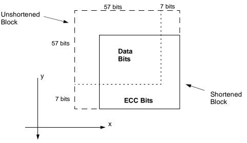
Figure 150—Structure of shortened 2 D block
