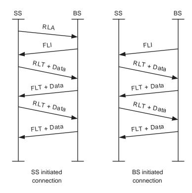
Figure 229—PHY control signal sequence diagrams
