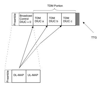
Figure 140—TDD downlink subframe structure
