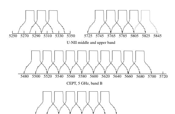
Figure 264—Channelization, 20 MHz
