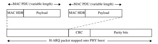
Figure 130—Construction of H-ARQ encoder packet
