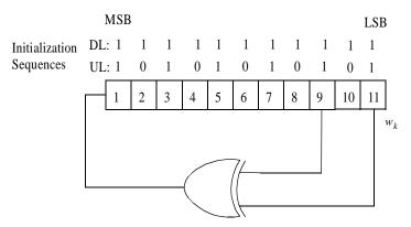
Figure 204—PRBS for pilot modulation
