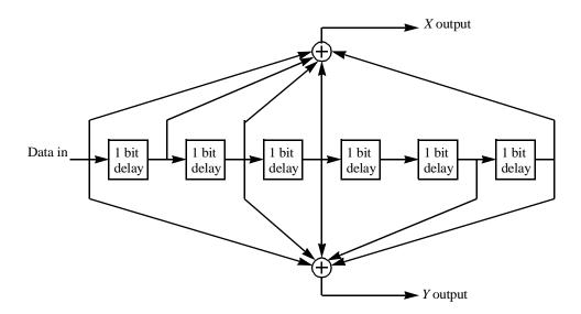
Figure 255—Convolutional encoder of rate 1/2
