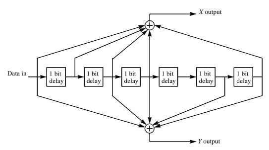
Figure 161—Binary rate 1/2 convolutional encoder
