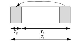
Figure 195—OFDM symbol time structure
