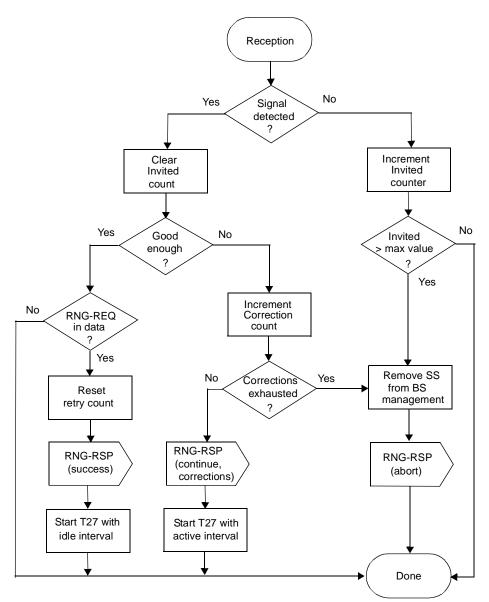
Figure 82—Periodic Ranging receiver processing—BS
