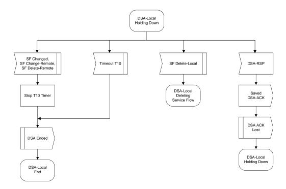
Figure 108—DSA—Locally Initiated Transaction Holding state flow diagram
