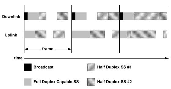
Figure 138—Example of FDD bandwidth allocation
