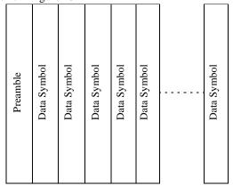
Figure 232—Downlink transmission basic structure
