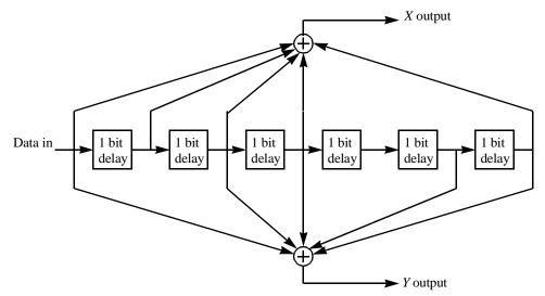
Figure 200—Convolutional encoder of rate 1/2
