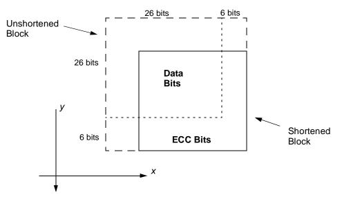
Figure 156—Structure of shortened 2 D block
