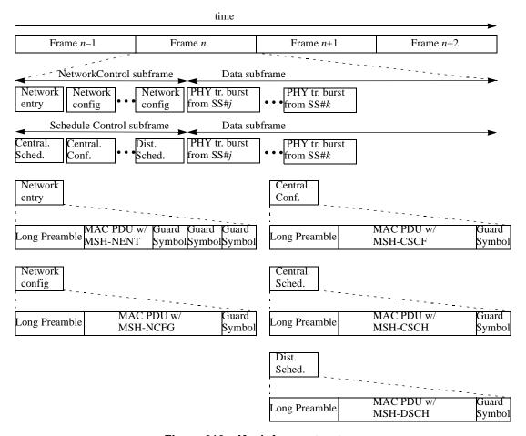
Figure 210—Mesh frame structure
