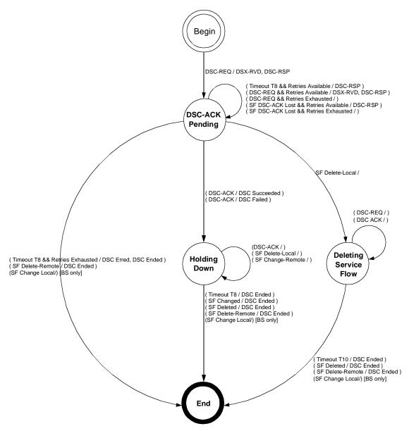
Figure 103—DSC—Remotely Initiated Transaction state transition diagram
