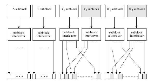
Figure 259—Block diagram of the interleaving scheme
