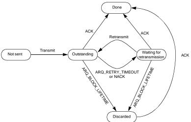
Figure 33—ARQ transmit block states
