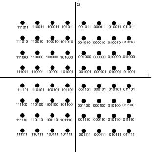
Figure 153—64-QAM constellation (gray-coded)
