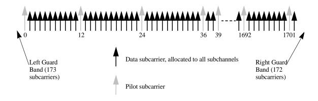
Figure 235—Downlink symbol structure for segment 0 on symbol number 1 using FUSC
