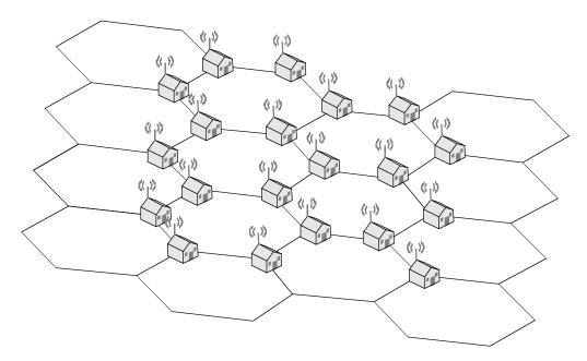
Figure B.1—WirelessHUMAN Mesh deployment model
