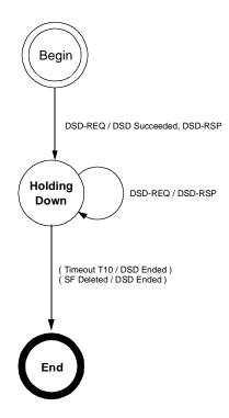
Figure 105—DSD—Remotely Initiated Transaction state transition diagram
