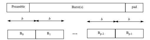
Figure 186—Base frame partitioning and padding
