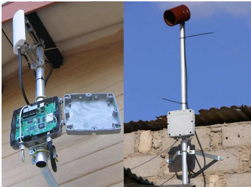
Figure 6.2: Outdoor mesh node with repackaged Linksys WRT54G electronics in a waterproof aluminium case. The picture on the left shows an installation at node D is using a commercial 8dBi flat panel, the picture on the right shows an installation at node H which is using a home made Cantenna.
